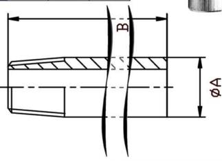
Our Threaded Fittings are produced through the castings process and can be supplied in material 316 with threads according to NPT and BSP.
