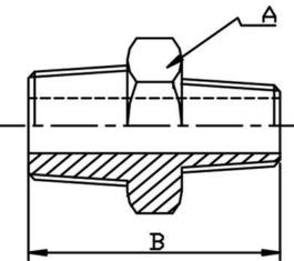
Our Threaded Fittings are produced through the castings process and can be supplied in material 316 with threads according to NPT and BSP.
