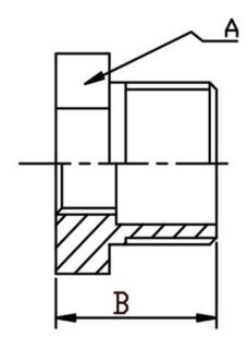
Our Threaded Fittings are produced through the castings process and can be supplied in material 316 with threads according to NPT and BSP.
